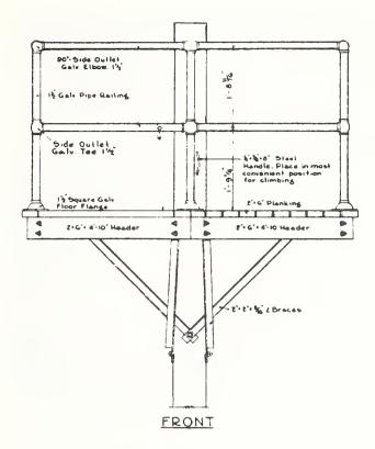
Figure 67. The "crows nest" detailed in plans for an "Observation mast for emergency lookout, 1937." These were to be only briefly occupied.
